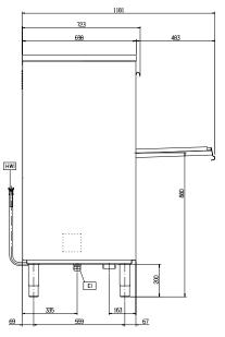
Drain EI = Electrical inlet (power) Electrical Outlet Hot water inlet Rinse aid connection XR
